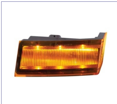
Item No. 36006 6 LED Amber Turn Signal Light For 2018-2023 Freightliner Cascadia - Driver - Competition Series MSRP: $ 39.99 OEM No. : A06-90212-002, A06-90212-005
